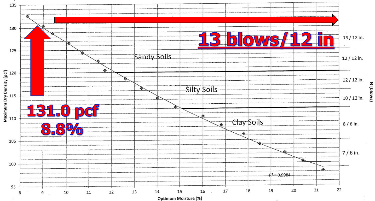
Maximum Dry Density - Optimum Moisture Content vs DCP Criteria
