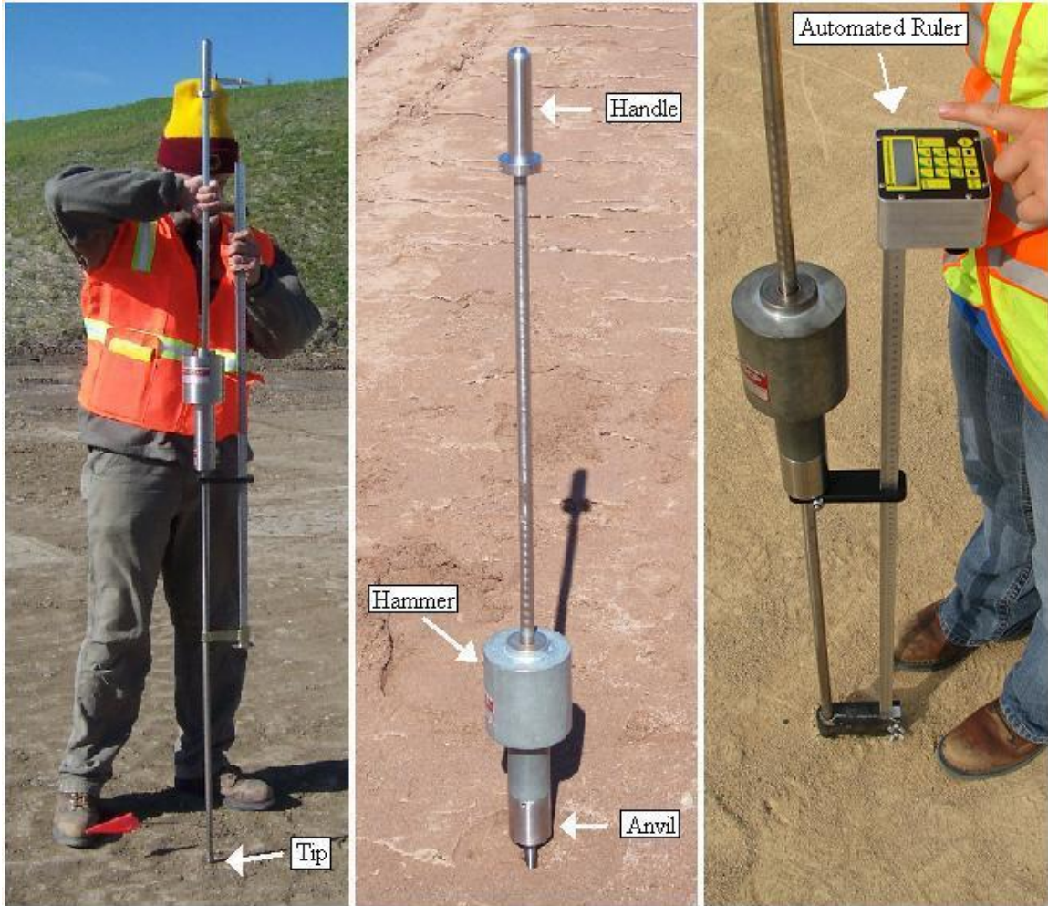
Figure 1.1. Photos of the dynamic cone penetrometer
